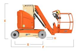
A. Platform Width 41.3-in / 1.05-m Platform Length 27.5-in / 0.70-m В. Machine Width 3-ft-11.25-in / 1.20-m 5.9-in / 15-cm Tailswing Machine Height 6-ft-6-in / 1.98-m Machine Length 12-ft / 3.65-m (Drop Bar) Wheelbase 5-ft 3-in / 1.60-m H. Ground Clearance 3.9-in / 10-cm
