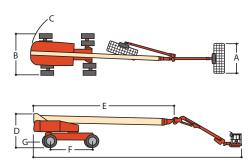
**Standard Features** Platform: 36 x 96 in. (0.91 x 2.44 m) Side Entry 8 ft (2.44 m) JibPLUS° Boom Selectable Capacity Envelope 180° Hydraulic Platform Rotator AC Receptacle in the Platform 5 Degree Tilt Alarm/Indicator Light All Motion Alarm Swing-Out Engine Tray 12V DC Auxiliary Power Hourmeter Control ADE® System Full-time 4WD 3 Selectable Steering Modes Drive-out Extendible Axles Oscillating Axle
